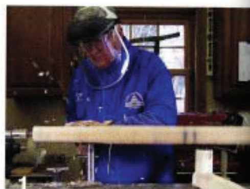
Mount a kiln-dried 2x2x37" blank between centers. (Hardwoods such as maple, walnut, oak, and ash work best.) Using a spindle roughing gouge, C. A. Savoy brings the bottom half of the cane into round by working from the tailstock toward the headstock.
